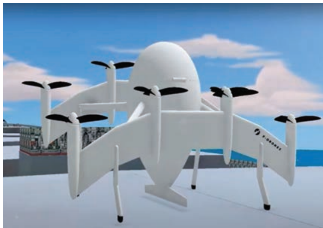
F-drones is developing a new drone technology that will be capable of delivering 100kg loads across a 100km range
